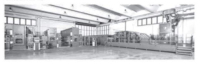
Another step to improve evenness is the card feeder MultiFeed designed by DiloSpinnbau which is available in working widths up to 5 m. This machine using the "Twinflow" infeed system offers a capacity of over 400 kg/hour/m of working width when processing 1.7 dtex fibres. It thus represents a state-of-the-art feeding solution for direct cards. The use of a "Twinflow" infeed applies the doubling effect for a more homogeneous flock mass flow.
